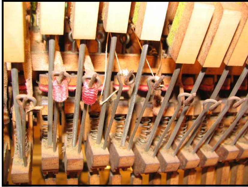
Mismatched or incomplete set of bridle straps.
