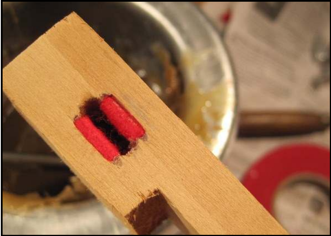
A key which has been professionally rebushed.
