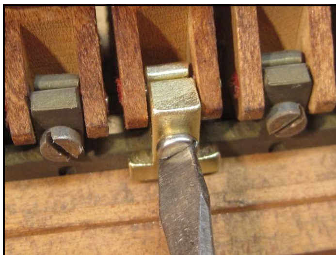
Repair clip for broken tongue being installed.
